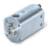
PulsaJet® electrically-actuated air atomizing spray nozzles provide high transfer efficiency to minimize waste and messy overspray. Cycle speeds up to 15,000 cycles per minute are possible to keep pace with fast line speeds. PulsaJet nozzles can be used with a variety of spray tips to ensure the performance matches the application requirements.
